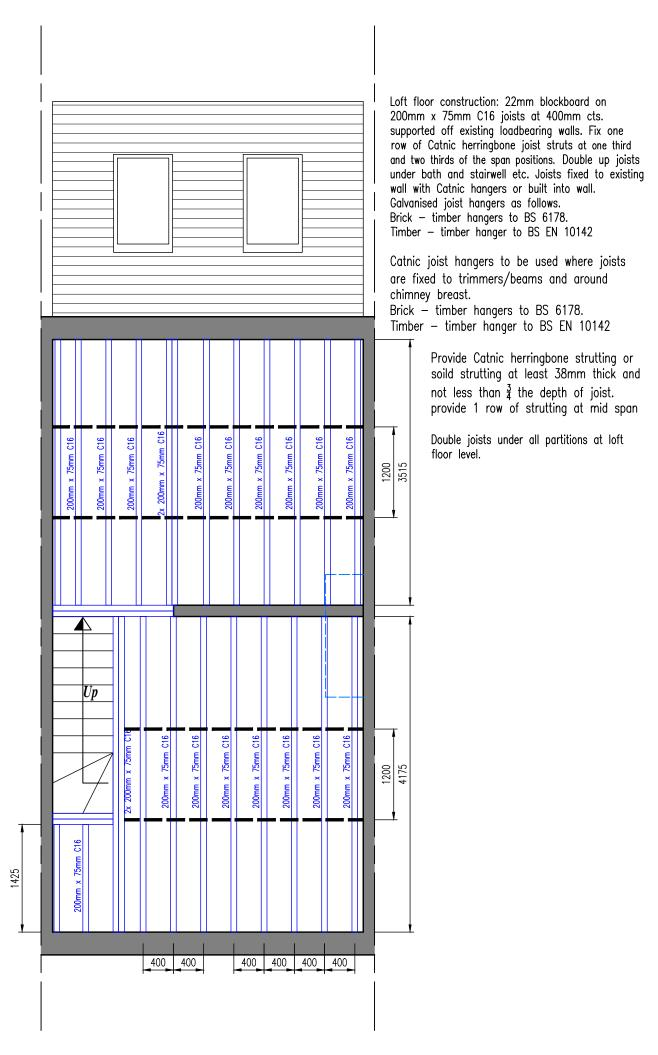
PROPOSED LOFT FLOOR JOIST PLAN scale 1:50
